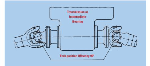
If two or more drivelines are arranged in series behind each other, it is recommended that they be mounted offset to each other by 90°. Doing so will at least partially cancel to the outside the effect of the mass acceleration forces caused by the fluctuation motion of the driveline center parts.
