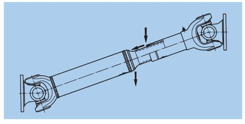
These drivelines should be arranged such that the spline, whenever possible, is protected from dirt and moisture. As a rule, this means installing the driveline according to the sketch above, where the spline seal points downwards so that spray water hitting it runs away from the spline.
